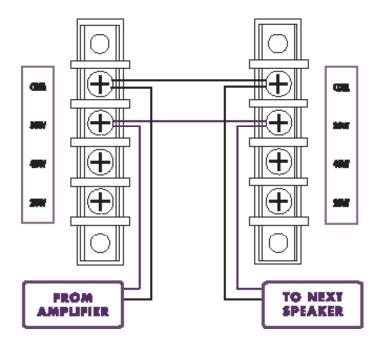
Select the power tap by dividing the amplifier's available power by the number of speakers to be connected. Always select the next lower wattage tap. For example:
